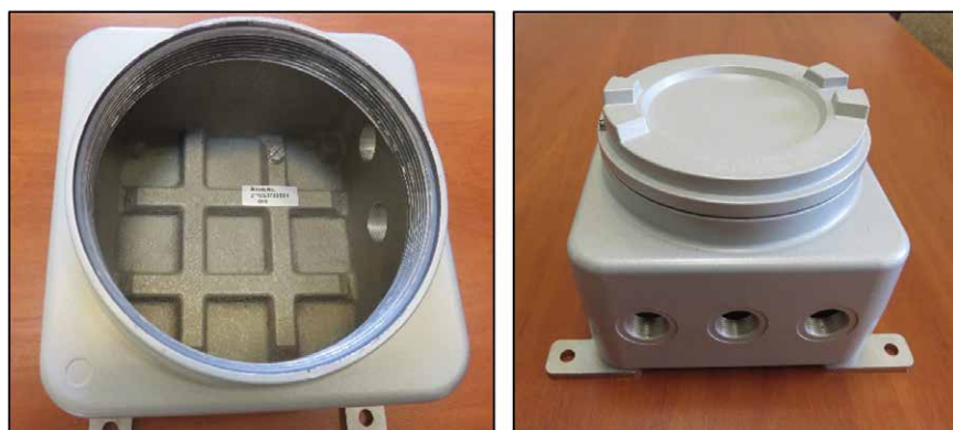
Fig. 13: Inner surface of the casting (explosion-proof instrument housing) after removing the coated sand core. (courtesy Limatherm S.A. Poland).
