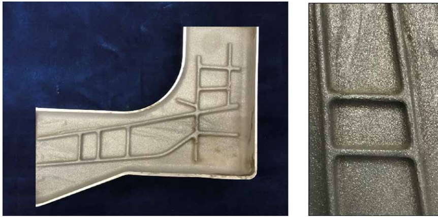
Fig. 16: Sand cores with a coating applied by dipping. The coating was furnace dried at 120 °C for 1 h.
