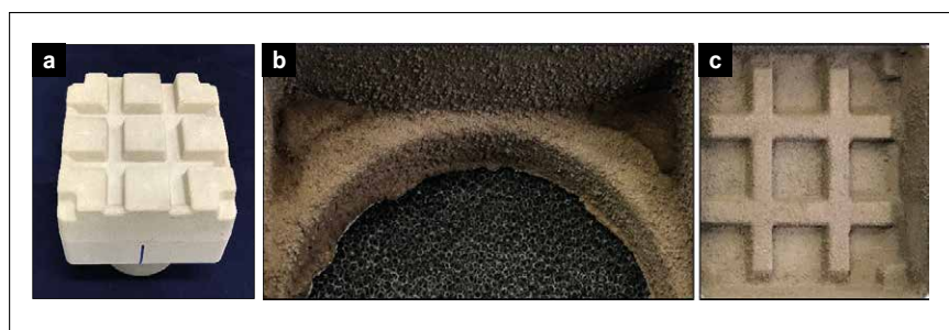
Fig. 11: Left: non-coated sand core; middle and right: inner casting surface with significant sand adhesion.
