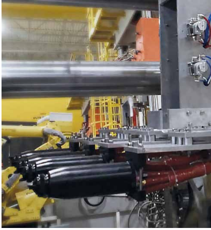
Fig 1: Effective minimum lubricant application with the Lubrolene spray head.
