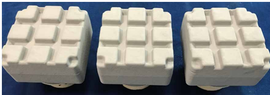
Fig. 12: Sand cores with a coating applied by dipping. The coating was furnace dried at 120 °C for 1 h.
